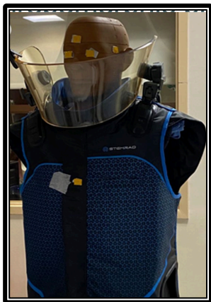
Interventionalist Mannequin 1a ) wearing novel radiation protection exoskeleton with tall visor setup ( short visor setup not pictured )
